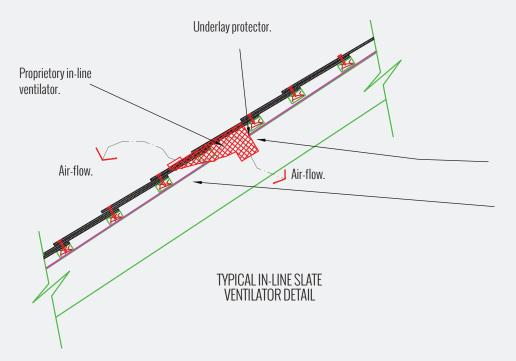
Cut slating batten and underlay locally to accommodate ventilator.
